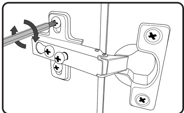
**EN** To move the door position left or right adjust as shown.
