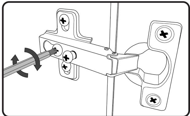
**EN** To move the door position up or down adjust as shown.
