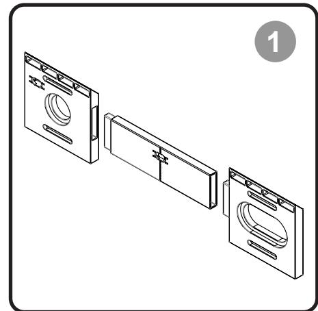
**EN** Once the bracket is assembled hold it against the wall surface where you intend to hang the product. Using a pencil, mark the screw hole positions through the template in each cam recess. Remove the template and Hang 'N' Lock bracket from the wall surface prior to drilling.
