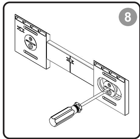
**EN** Fit the cabinet onto the Hang 'N' Lock bracket. Secure in position by inserting the two locking studs through the holes inside the cabinet. Rotate the studs 90 degrees clockwise to lock into position.
